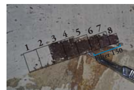
Fig. 4 EOS1000 LQS trials on wet surface. 1) 0.44 J/cm²; 2) 0.63 J/cm²; 3) 0.99 J/cm²; 4) 2.54 J/cm²; 5) 3.98 J/cm²; 6) 0.49 J/cm²; 7) 0.88 J/cm²; 8) 1.27 J/cm².
