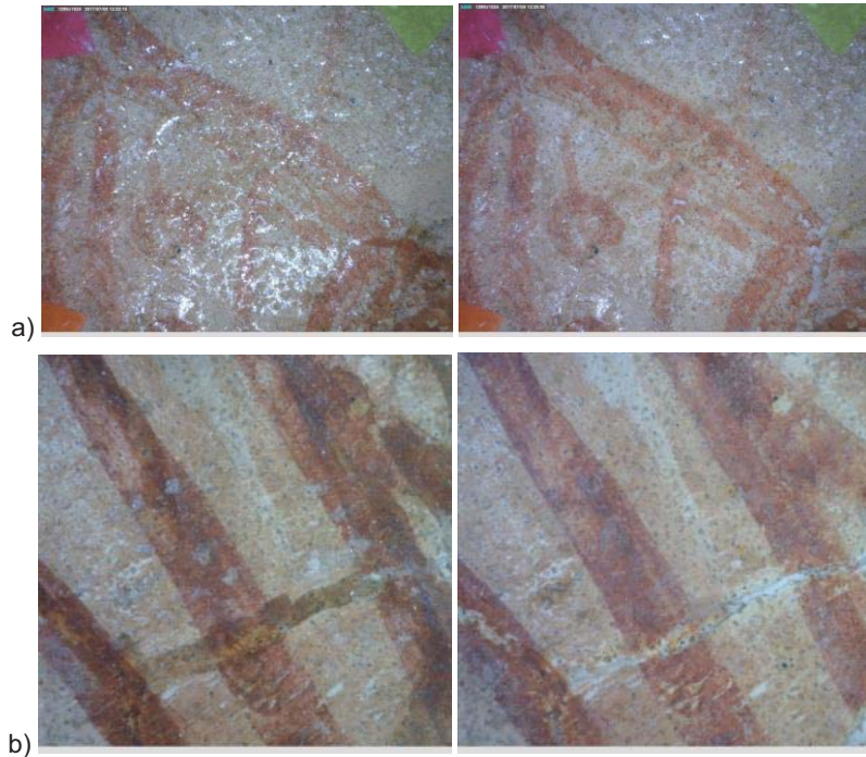
Microphotographs of the painting surface during laser trials before (left) and after (right) the laser removal of a) coating and b) overpainting.
